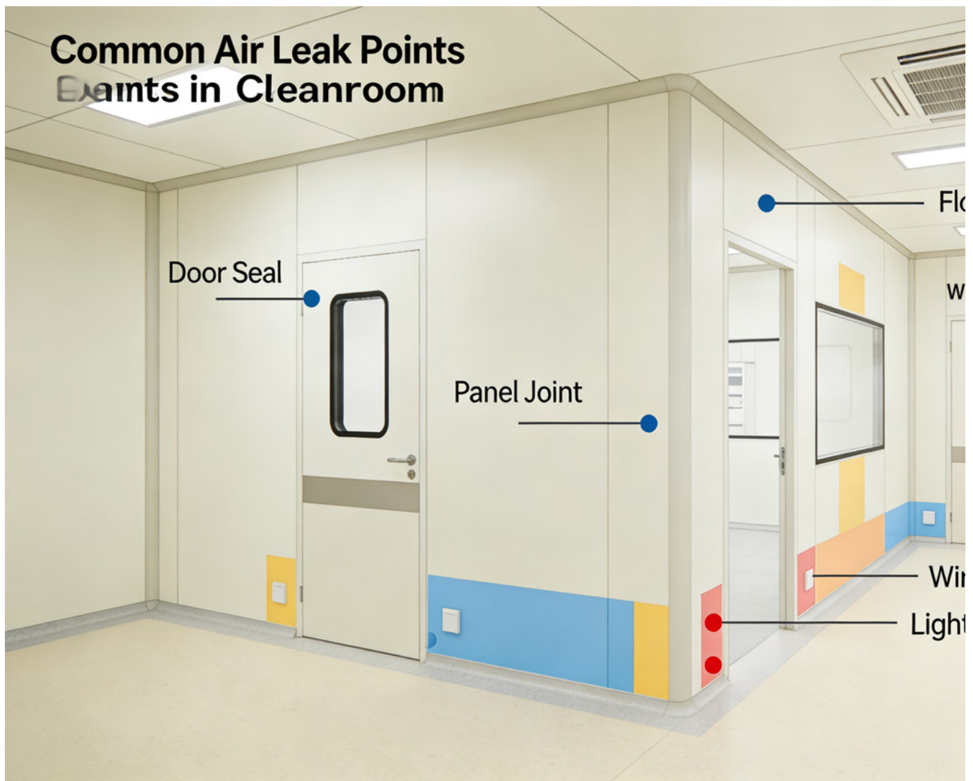
Typical air leakage locations in cleanroom enclosures
